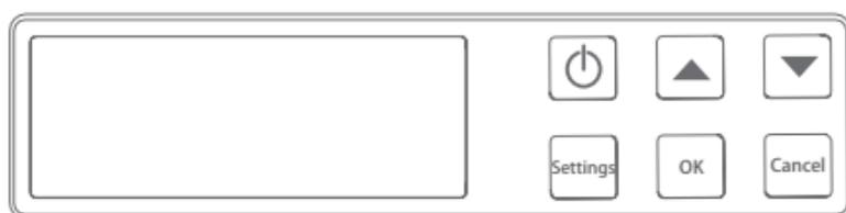
**ON/OFF button:** Press the ON/OFF button to turn on the XStation. Press and hold it for at least 5 seconds to bring up the shutdown/restart menu. Press the Select buttons to select the operation required and then press OK.
