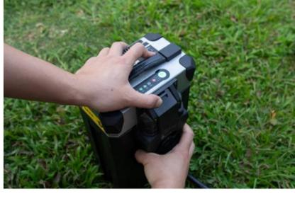
⚠ DO NOT disconnect the battery when it is ON, otherwise the connector may be damaged
