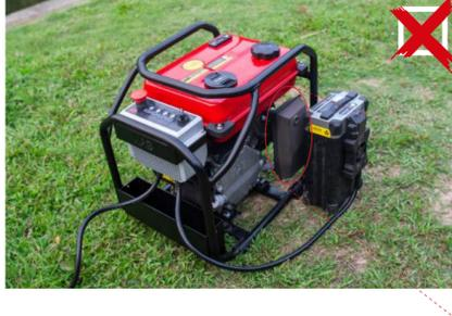
⚠ Keep Battery away from muffler to avoid damage to the battery due to high temperature.
